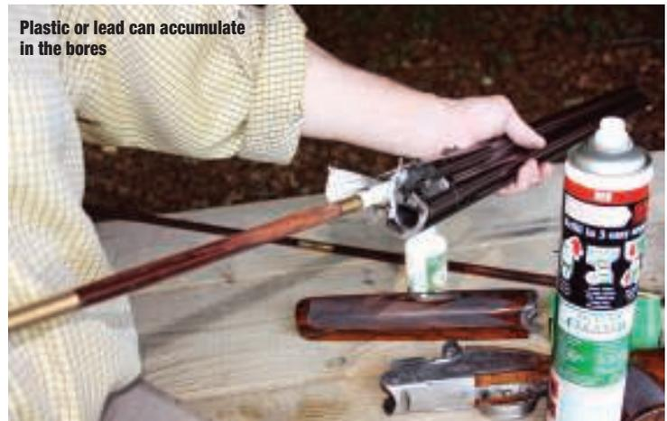
Plastic or lead can accumulate in the bores
