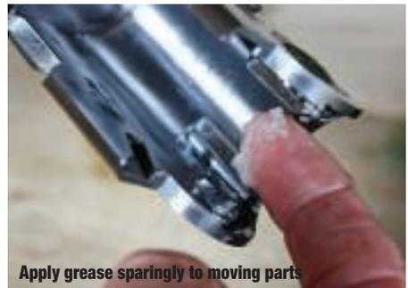
Apply grease sparingly to moving parts
